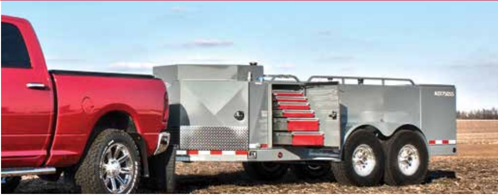
Above (from left): LDJ workers prep a trailer before it enters the state-of-the-art paint facility; ASME-certified welders manufacture tanks to be used on fuel trailers; and a 750 Gallon Service Special trailer that transports diesel fuel, diesel exhaust fluid, and oil including room for tools and parts.
